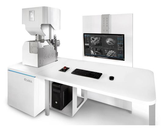
TESCAN CLARA - Field-Free analytical UHR SEM for materials characterization at nanoscale
