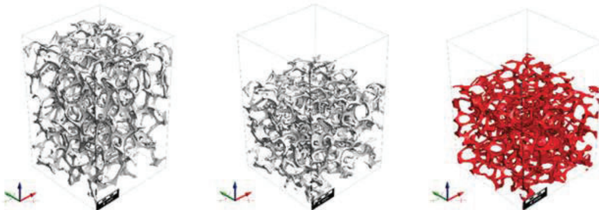
FIGURE 3 Left + middle: segmented datasets from the dynamic micro-CT experiment at 0 and 35% compression. Right: Simulated sample at 35% compression.
